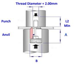
Punch Or Drill Hole To Specified Diameter (DO NOT Deburr The Hole Seat Fastener Squarely In The Hole
